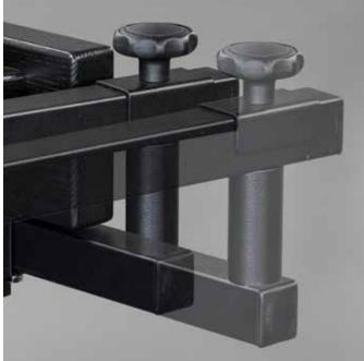
Gas tubes make for effortless height adjustments. The desired height can be locked into place using a spring loaded pin and wingnut. Additionally, the height adjustment tubes are lined and numbered to help easily replicate setup and ensure both sides are set evenly.
